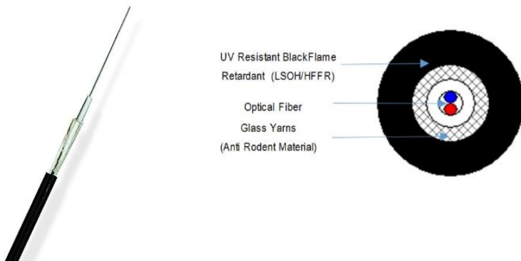
Gambar 2.6. Kabel Dalam Ruangan (Indoor Cables) FTTH Loose Tube Design (CCSI Standard Design Cables)[7]
