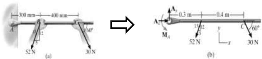
Gambar 4.7. Uraian diagram benda bebas Sumber : Engineering Mechanics
