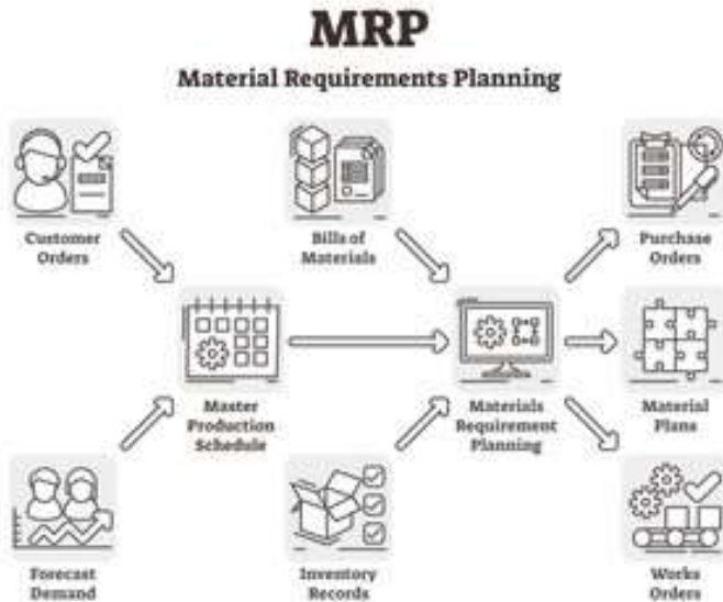
Gambar 11.34. Material Requirement Planning cycle *Sumber Sutterstock.com
