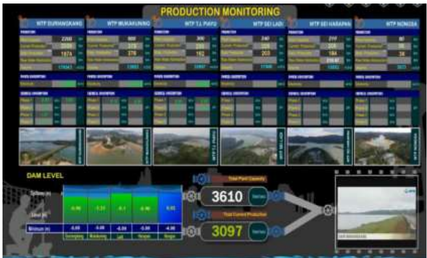
Gambar 10.3 : SCADA –DASHBOARD Production Monitoring (Sumber: perpamsi.or.id, 2017)
