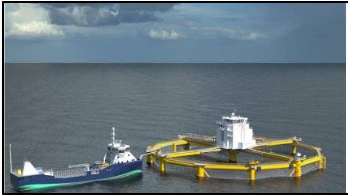
Gambar 10.4. Sistem KJA Lepas Pantai tipe Semisubmersible Offshore Aquaculture ( www.maritime-executive.com dikutip dalam Purnawanti, 2018)
