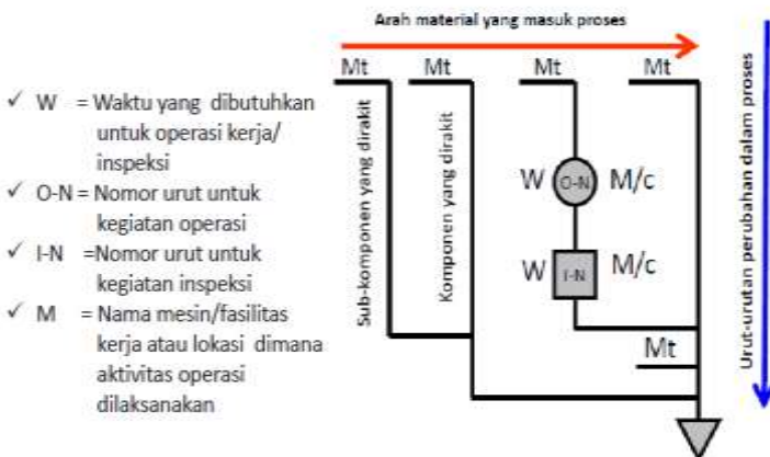
Gambar 12.1. Aturan Umum Membuat Operation Process Chart Sumber : Iftikar, 2006
