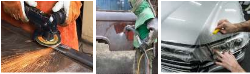
Gambar 35. Proses Oprasi Permukaan (Surface processing operations): a) Pembersihan (cleaning): Proses Grinding; b) Perlakuan permukaan (Surface treatments): Proses Sand Blasting; c) Proses pelapisan dan deposisi film tipis (Coating and thin film deposition): Proses Coating Film.
