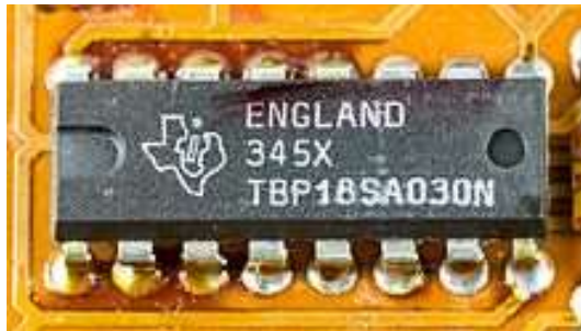
Gambar 4.3 : Chip PROM Texas Instrumen TBP18SA030N Sumber : wikipedia.org
