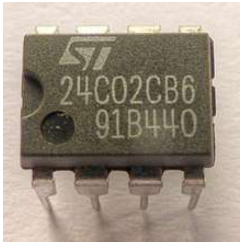
Gambar 4.5 : Chip EEPROM STMicro M24C02 Sumber : wikipedia.org
