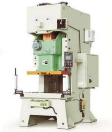
Gambar 5.9. Mesin Stamp Vertikal (Stamping Machine). (Sumber: sunrui)
