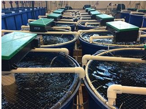
Gambar 7.8. Sistem Recirculating Aquaculture System (RAS) Sumber: https://en.wikipedia.org/wiki/Recirculating_aquaculture_system
