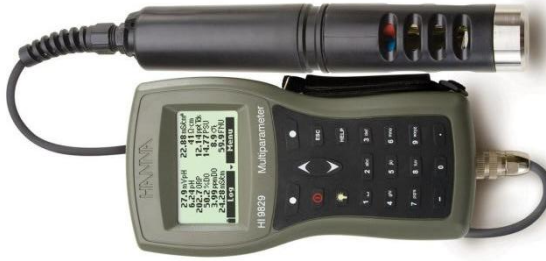
Gambar 4.13. Multiparameter probe HI98194 (Sumber : hannainst.com.au)
