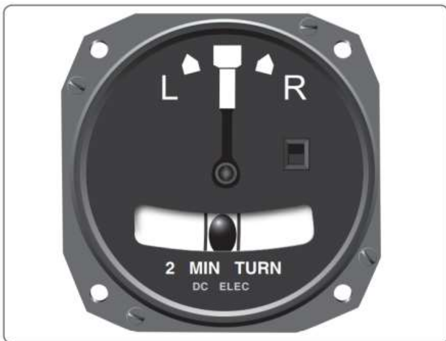
Gambar 2.88. Indikator belok dan geser tampak depan (Sumber: [U.S. Department of Transportation, 2012])
