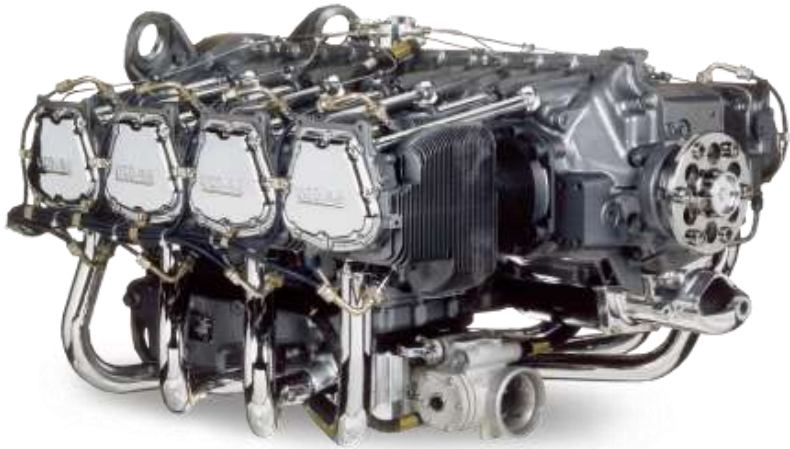
Gambar 8.105. Mesin penggerak piston 8 cylinder Horizontal (Sumber : Lycoming)
