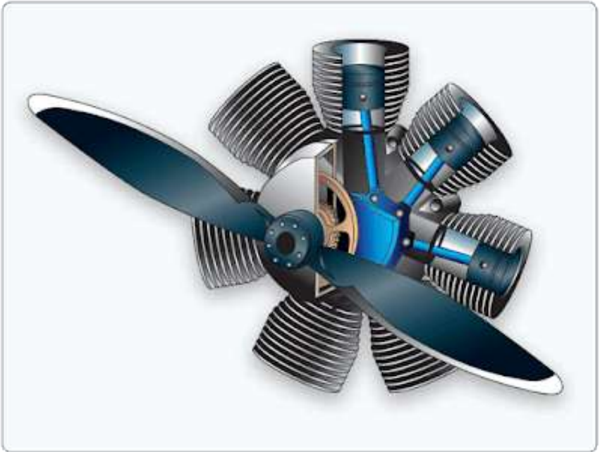
Gambar 8.108. Mesin radial 6 silinder (Sumber : Flight-Study.com)
