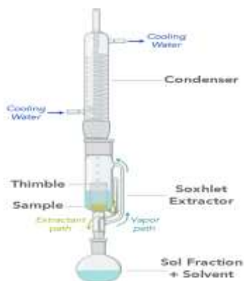
Gambar 3.4. Soxhletasi (Sumber :Danielsen et al. , 2021)
