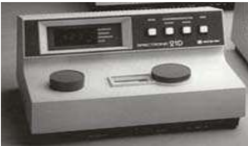
Gambar 13.2. Alat Spektrofotometer UV-VIS Single-Beam (Spectronic-20). (Sumber: (Dachriyanus, 2014))
