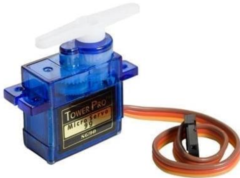
Gambar 4.5. Motor servo (Sumber : Prastyo, 2022)
