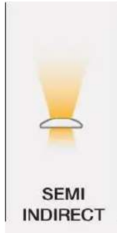
Gambar 5.3 Semi Indirect Lighting
