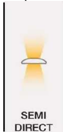
Gambar 5.4 Semi Direct Lighting
