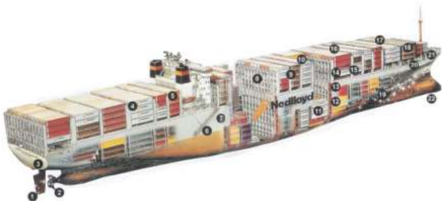
Picture 3.12. Open Container Vessel (van Dokkum, 2011)
