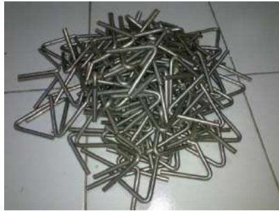
Gambar 4. 8. Anchor V Shape
