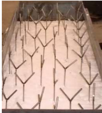
Gambar 4. 9. Anchor Y Shape
