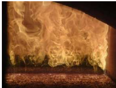
Gambar 5. 1. Refractory dry out
