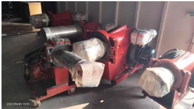
Gambar 5. 4. Contoh Burner External
