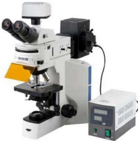
Gambar 4.7. Mikroskop Fluorescence (Sumber : Bidlack dan Jansky, 2011) Alponsin, 2019)
