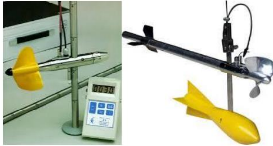
Gambar 7.7. Current meter horisontal (tipe baling-baling) (P3SDA)
